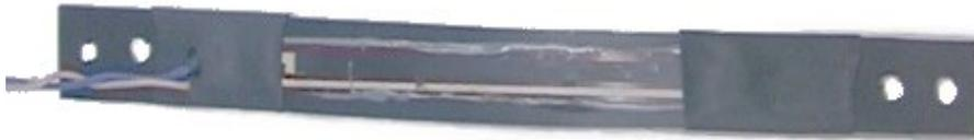
Figure 8.5: The finalized sensor design.
