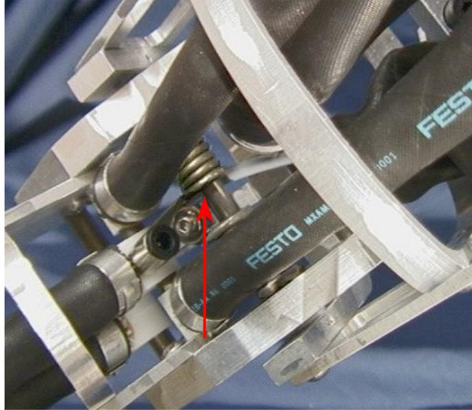
Figure 2.4: Close up of a middle leg coxa-femur joint on Robot V. The arrow points to a torsion spring.
