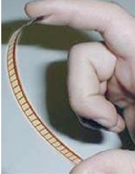
Figure 8.1: Spectra Symbol flex sensor.
