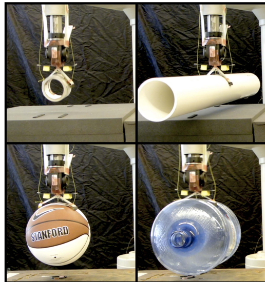
Fig. 17: Objects picked and placed by a robotic arm using the shear adhesion gripper. Clockwise, from upper left: packing tape, PVC tubing, 5 gallon water bottle, and basketball.
