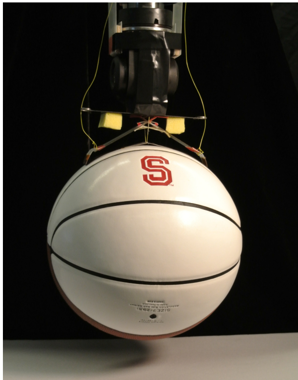
Fig. 1: Shear force gripper holding a regulation-size basketball.
