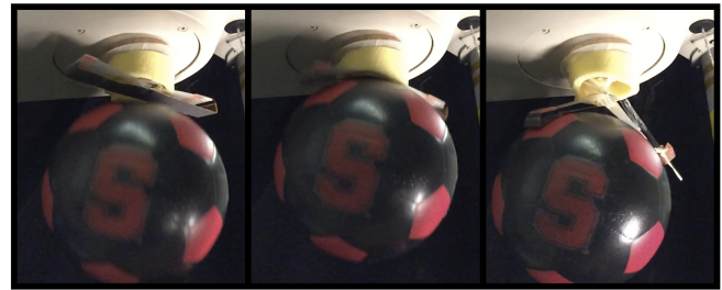
Fig. 18: Gripper catching a ballistic object. Left , The instant before contact is made ( t = 0 ). Center , The gripper collapses ( t = 20 ms). Right , The ball rebounds, but the adhesive has engaged, and the gripper has caught the ball ( t = 88 ms).
