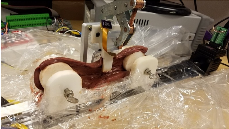
Figure 5.4 – Benchtop experiment setup for prototype slip sensor validation, shown holding slice of liver tissue. Data used in publication reflects experiments on turkey bacon, rather than liver as shown here.
