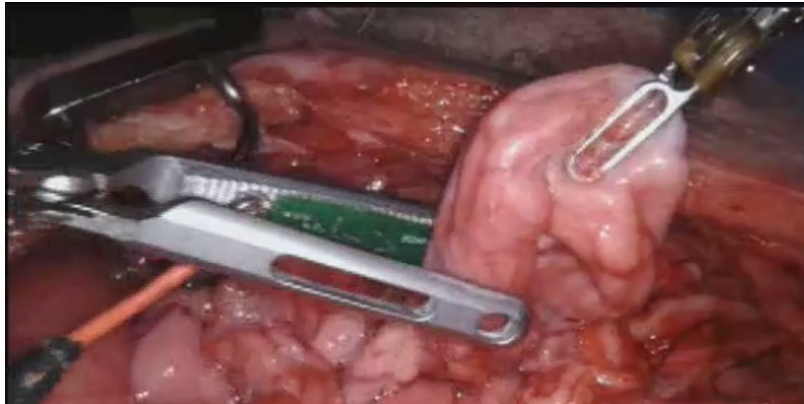
Figure 5.19 – In vivo porcine testing via laparotomy and da Vinci Xi Surgical System with prototype grasper (left hand) and Fenestrated Bipolar Forceps (right hand).
