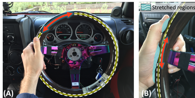
Fig. 1. (A) Skin stretch steering wheel display: ring at front of the rim shown in yellow highlighted region with dotted line can rotate \pm 0.5 degrees, producing \pm 2.5 mm of skin stretch, and can be gripped anywhere. Integrated motor is visible at the 5 o'clock position. (B) Close-up view of the skin stretch. The palm and thumb pad are the most likely areas to be stimulated.
