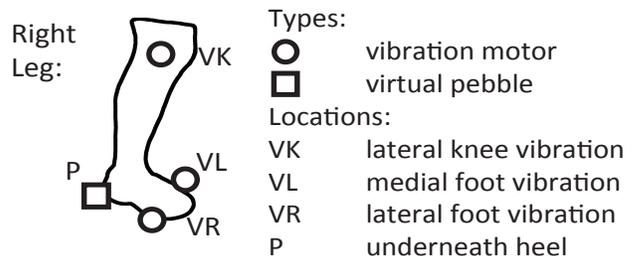
Fig. 3. Symbols and abbreviations for haptic feedback types and locations
