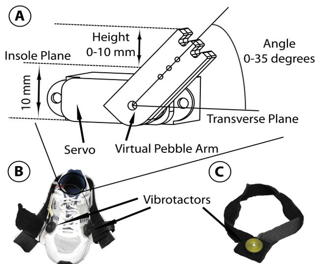
Fig. 1. The virtual pebble (A) consists of a small servo motor and a rotating arm ( $20.3 \times 7.6 \times 4.6$  mm), embedded in the heel of the shoe (B). Two vibrotactors (C2 factors) are attached to the outside of the shoe and one to the outside of the knee via Velcro straps (B), (C).
