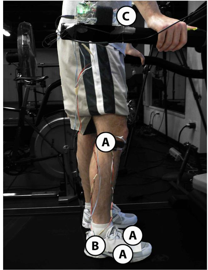
Fig. 2. Experimental setup showing a subject standing on the treadmill with three vibrotactors (A) attached to the knee and foot and one virtual pebble (B) underneath the heel. A microcontroller (C) receives heelstrike signals and controls the haptic actuations.
